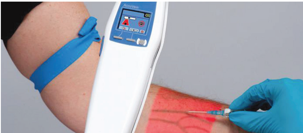
Figure 1 The AccuVein AV400 device uses red and infrared reflection to detect the haemoglobin in the vessels 10
